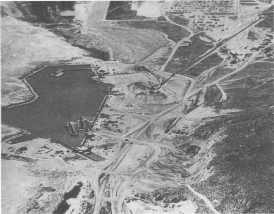
An aerial view of Little Valley and its “sea port” which was built to provide rock and gravel fill for the railroad causeway built across the Great Salt Lake 1956–1959. (Box Elder County)
